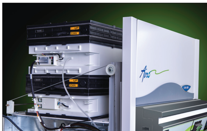
The 3' Protector Airo Filtered Fume Hood with 31.7" depth uses two Neutrodine Carbon Filters, accessible from the side. Neutrodine Filters in 3' and 4' Protector Airo Hoods with 37.7" depths are accessed from the front. An optional HEPA Filter is available as an add-on to handle applications involving nuisance dust or powders.
