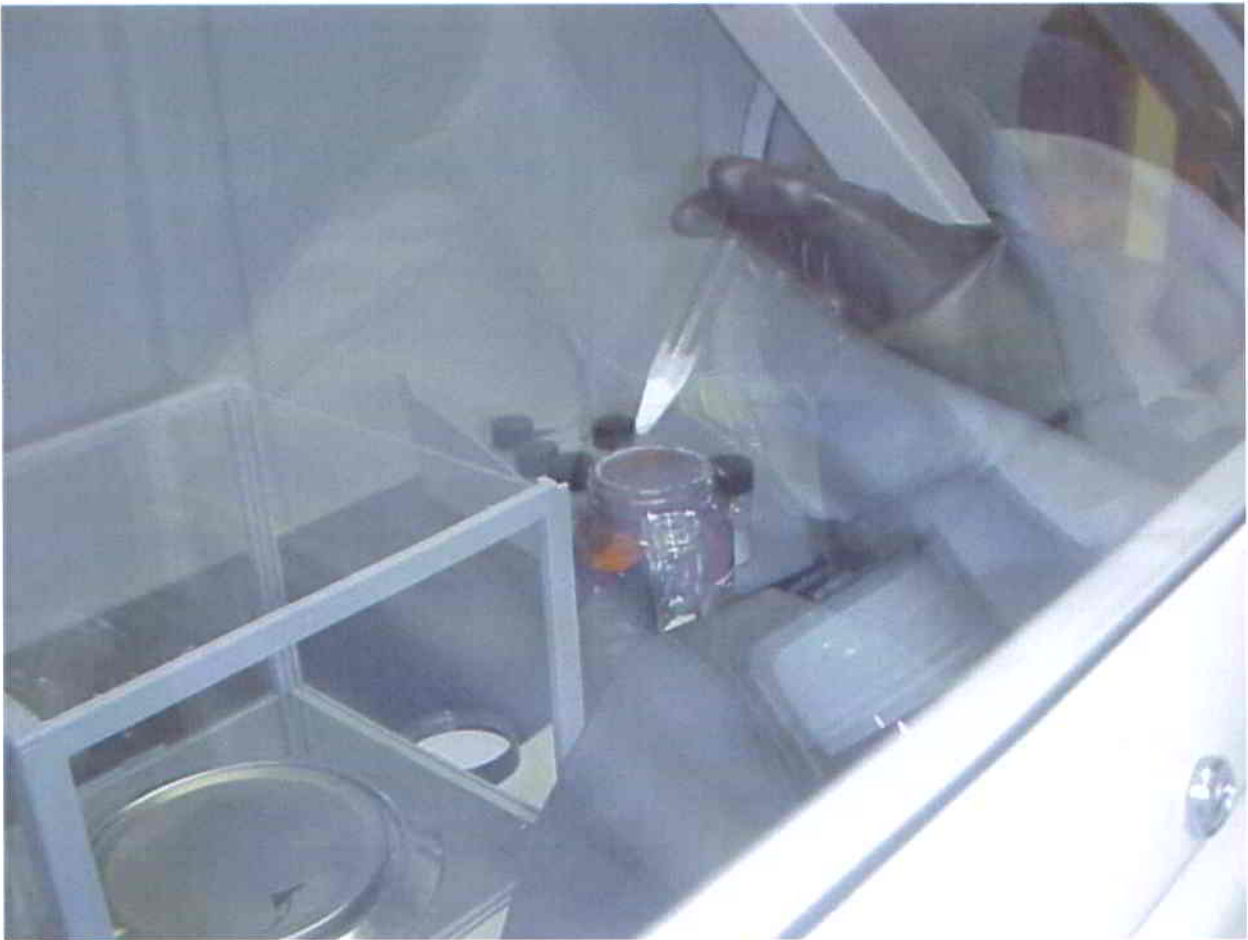
Operator #2 Weighing Technique (note wet towels to contain spills)
