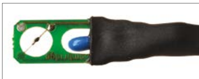
Figure 1. In biosafety cabinets using sensor-based airflow control, a thermal anemometer measures the downflow velocity in a single spot in the work surface.
