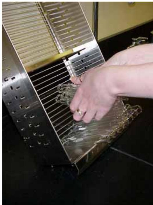
The tabs on the divider plate are inserted into the slots even with the level of
