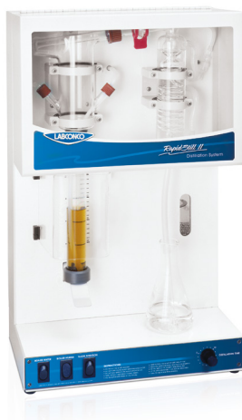
The RapidStill I is a steam distillation apparatus.
